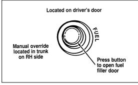
The remote control fuel filler door release button
